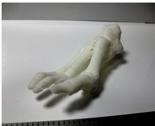
Figure 6.16 The generation of the whole foot structure, this was 3D printed from PCL biocompatible monomer.
