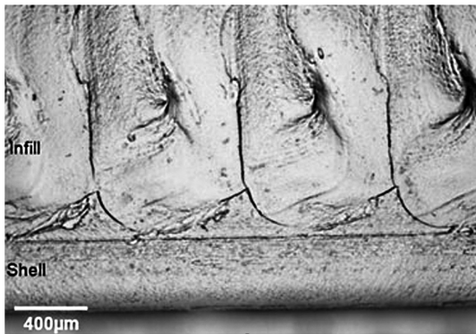
Figure 3.6 The two most critical factors to control carefully in 3D Printing are the layer resolution and the deposition of the exterior shell. It is these two significant properties which controls the edge and surface accuracy.
