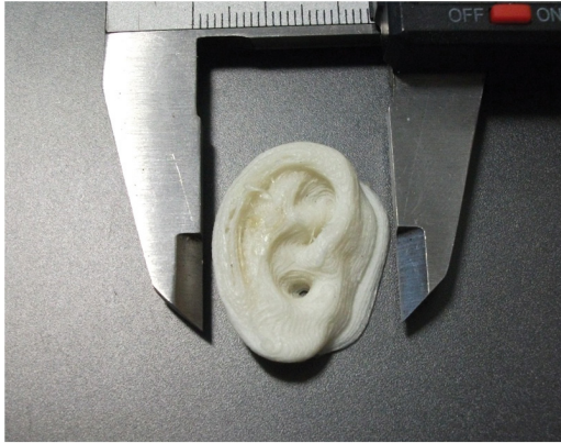
Figure 6.7 Coarse 3D printed structure of a young child's year model. This model has been produced from a latex polymer to mimic the flexibility of the original ear.
