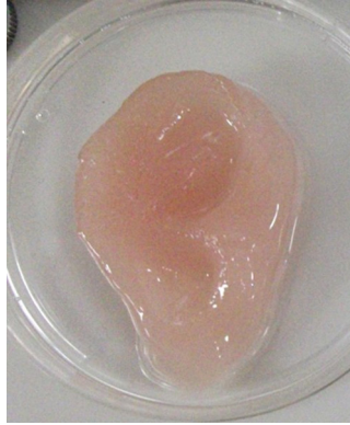
Figure 4.9 A photograph of a natural ear prosthetic device 3D printed from PDMS with the correct color and texture match.
