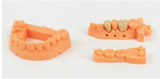
Figure 7.8 Dental model fabricated using the Continuous Liquid Interface Production (CLIP) methodology of 3D printing developed by Carbon3D Inc.
