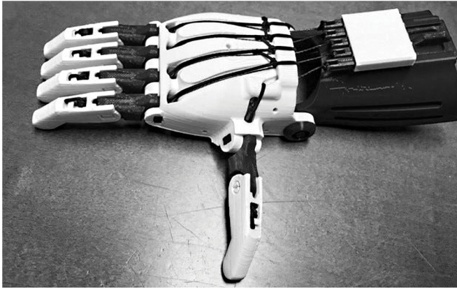
Figure 4.4 A 3D printed bionic hand with integrated finger positioning technology. Here, the device is fully open, however, each figure can be controlled independently.
