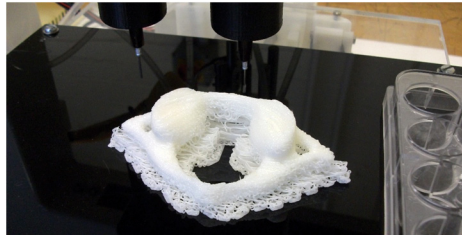
Figure 3.17 3D printed experimental water-soluble structure that is being testing to determine structural degradation.
