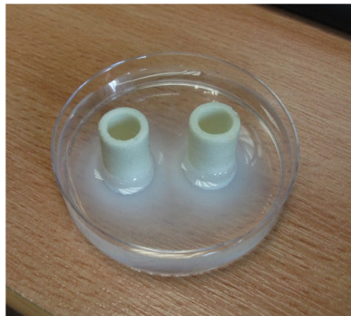
Figure 6.8 The fabrication of soft tissue models 3D printed from polyurethane and used for the purpose of surgical planning.
