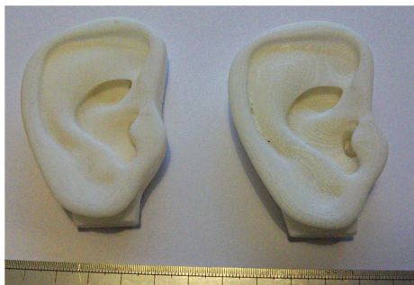
Figure 3.2 3D printed surgical models of the ears. Each was 3D Printed from Poly-Lactic Acid (PLA) and each small model took 2 h to 3D print.
