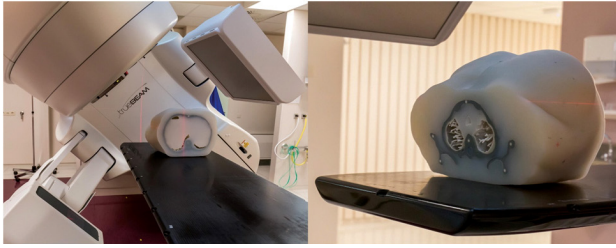
Figure 13.2 Experimental setup of phantom measurement for airway cancer treatment. Source: Reproduced with permission from ref [11].
