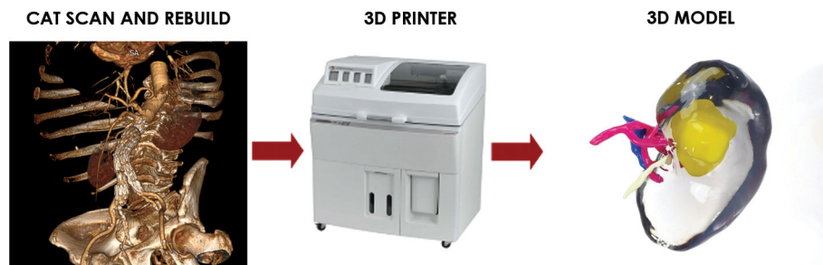
Figure 3.4 The process through which 3D Printed parts are created from patient data.
