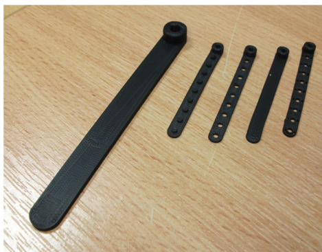
Figure 6.2 A series of 3D printed orthopedic fixings produced to suit the size required. Each is FDM 3D printed from carbon fiber reinforced Nylon 645.
