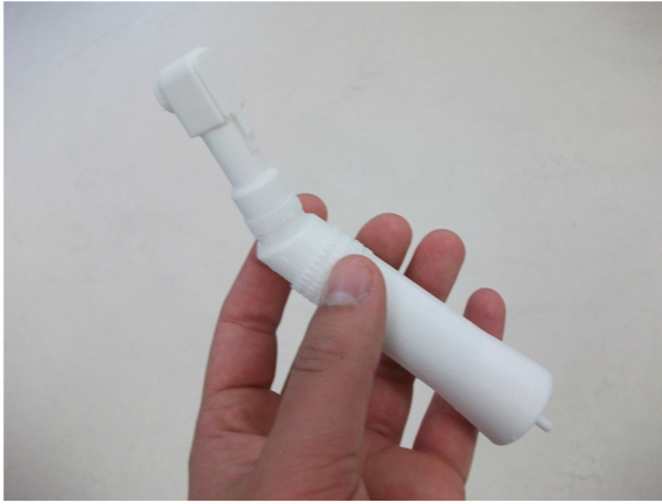
Figure 6.1 3D printed prototype dental surgical instrument that is 3D printed from HIPS.
