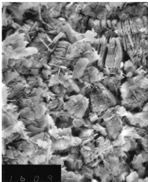
Fig. 32. Scanning electron micrograph of Belitung kaolin.
