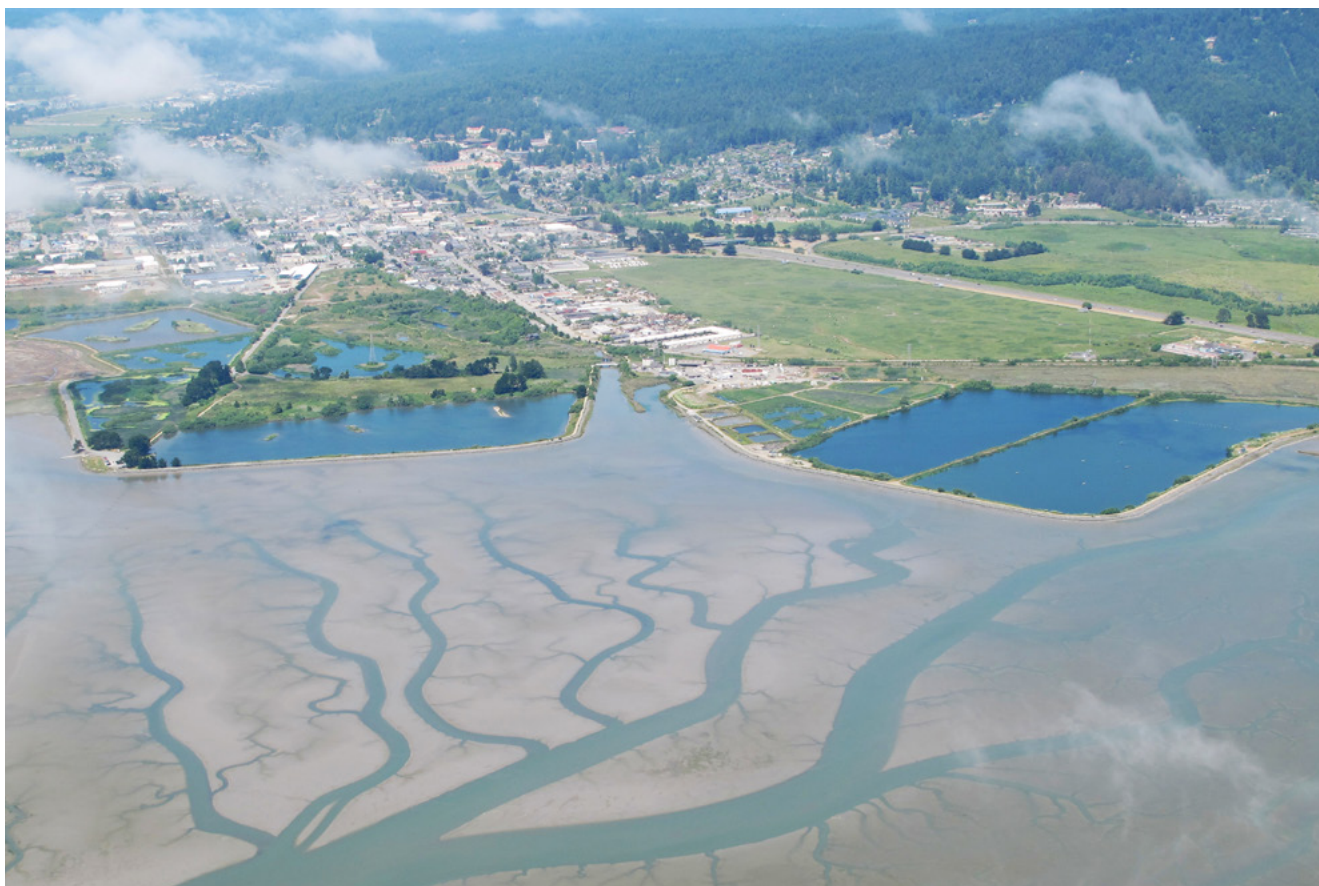
Figure 1: Arcata wastewater treatment plant, wetland system, and wildlife sanctuary on the edge of Humboldt Bay. Oxidation ponds and TWs on the right; enhancement wetlands and estuarine lake on the left; two urban streams enter the bay surrounding the site.
