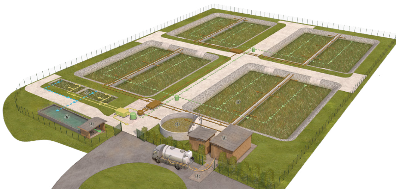
Figure 3: Schematic illustration of the Nègrepelisse septage treatment unit (source: Syntea). (1) A septic tank emptying place, (2) a stone trap followed by automatic screening, (3) an aerated buffer tank, (4) eight STRBs, (5) two VFTWs, (6) a storage basin of treated leachate, and (7) a filtration unit for irrigation.
