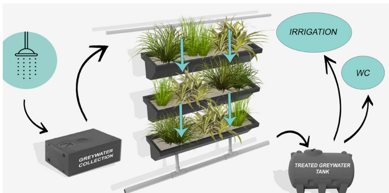
Figure 3: Schematic representation of the green wall of Margarita Beach, Ragusa
