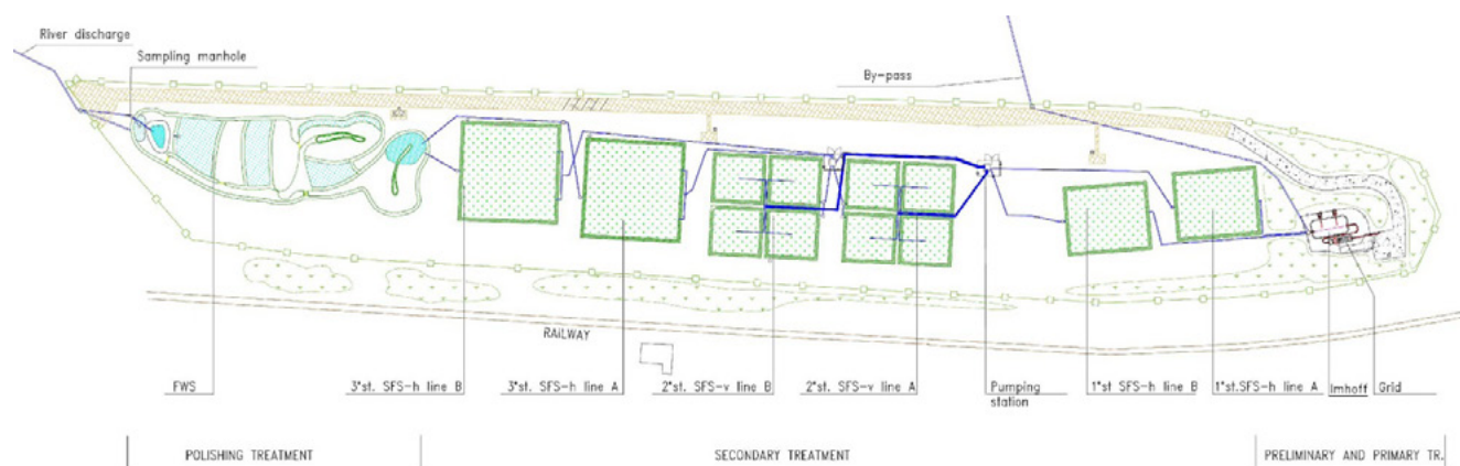
Figure 3: Schematic representation of the Dicomano TW WWTP; from Masi et al., (2013)
