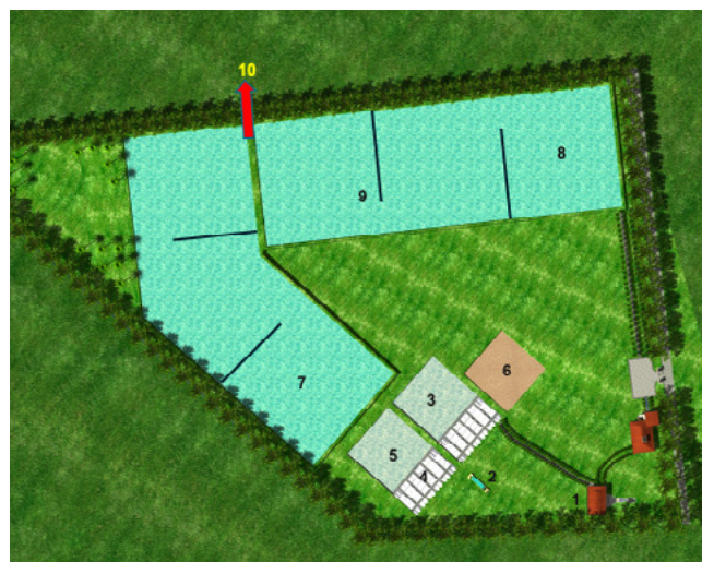
FIGURE 3: Design schematic of El Cerrito NBS-WTP. Source: Cinara (2003)
