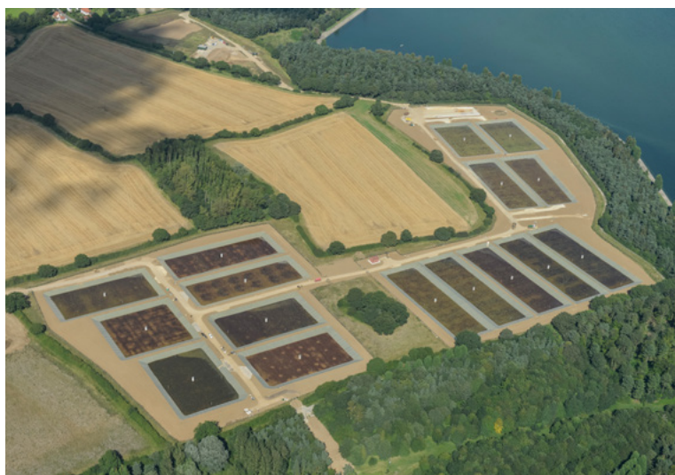
Figure 2: Hanningfield STRB; overview, sludge loading and sludge residue
